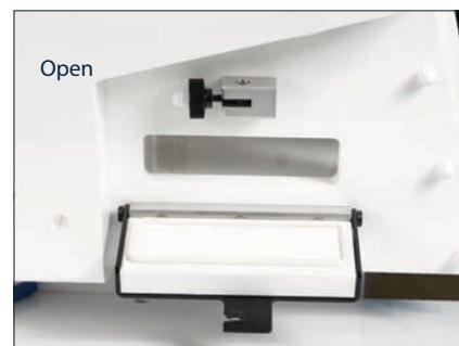
*Single plate entry system – allows quick entry or exit of individual plates.*
