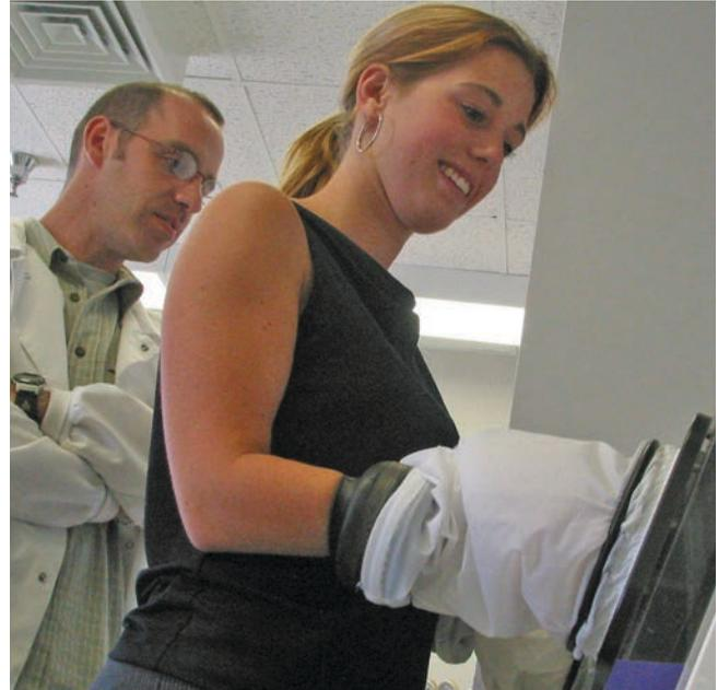
*Ezee Sleeve™ entry system provides access in seconds without disrupting the workstation atmosphere.*
